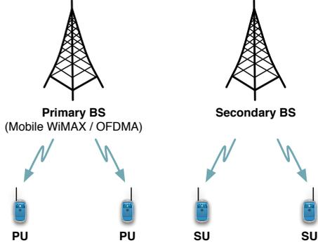
Fig. 1. The coexistent of primary and secondary systems
