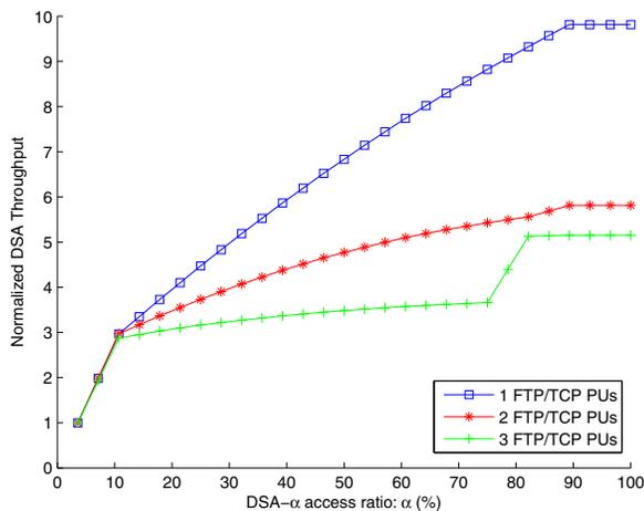
Fig. 7. Normalized Throughput in DL-Subframe: FTP/TCP Traffic
