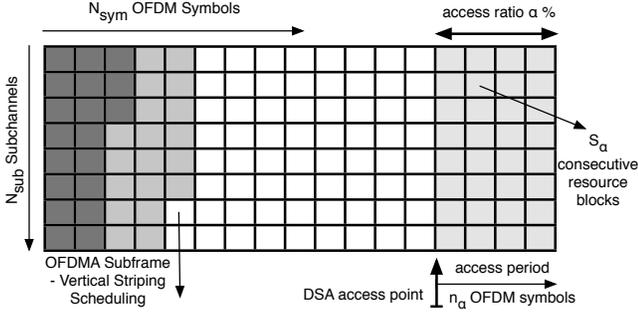
Fig. 3. Illustration of our DSA- $\alpha$  scheme in an OFDMA subframe
