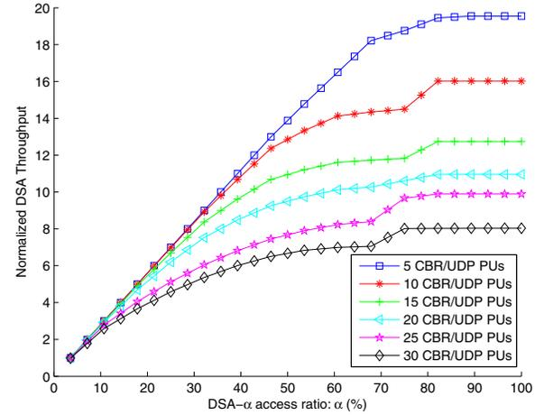
Fig. 5. Normalized Throughput in DL-Subframe: CBR/UDP Traffic
